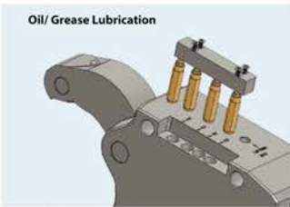
Oil/ Grease Lubrication
